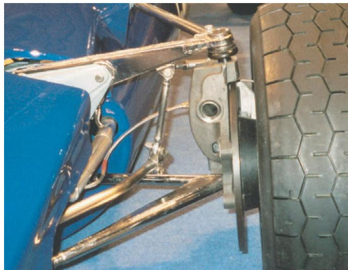
For motor cycles Rod Ends and Spherical Plain Bearings are used as stabilizers, for rod linkages and steering devices.
