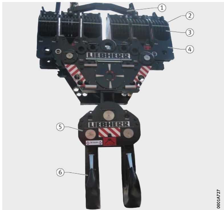
Figure 1 Modular design of hook block in fully assembled state
