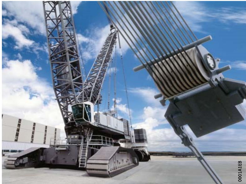
Figure 1 Rope sheaves in the Liebherr crawler crane
