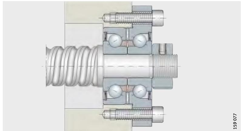
**Seals** Bearings with the suffix 2RS have lip seals and highly effective sealing. Bearings with the suffix 2Z are sealed using gap seals and are suitable for higher speeds.
