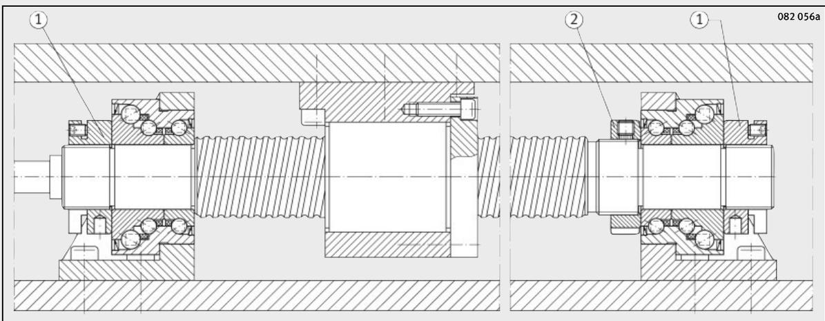
Ball screw drive spindle with locating bearing arrangement on both sides
