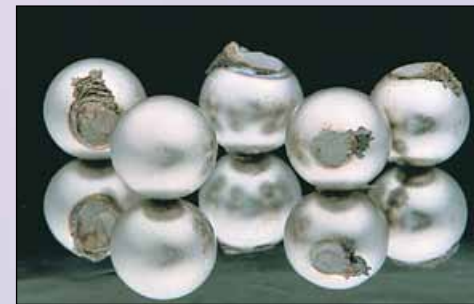
The above photograph shows the wear on 5 balls representing various different lubricants used during the test. The second ball from the left virtually unscathed, illustrates the use of Bardahl additives.
