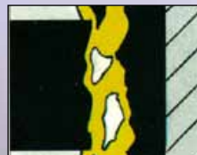
3 Molecular attraction between the hot bare metals can cause surfaces to tear against each other causing wear and eventual seizure.
